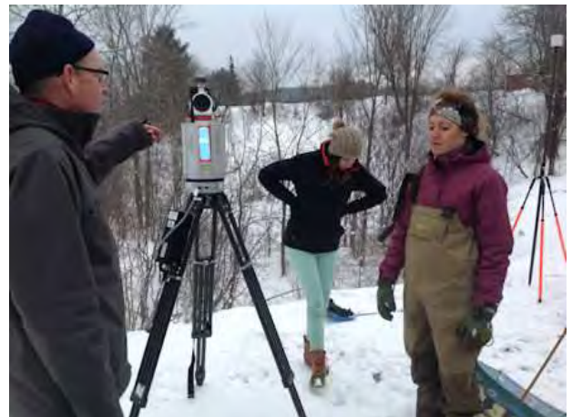
UVM Engineering students set up the LIDAR scanning equipment to capture a 3D image of the structure. (Image property of VTrans)
